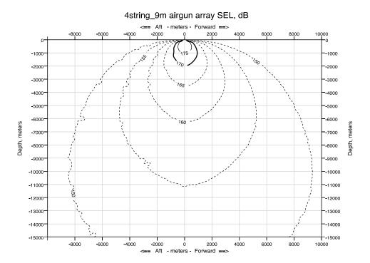
FIGURE A1. Modeled deep-water received sound levels (SELs) from the 36-airgun array planned for use during the survey, at a 9-m tow depth. Received RMS levels (SPLs) are expected to be ~10 dB higher. Plot at the top provides radius to the 170 dB SEL isopleths as a proxy for the 180 dB RMS isopleths and plot at the bottom provides radius to the 150 dB SEL isopleth as a proxy for the 160 dB RMS isopleth.
