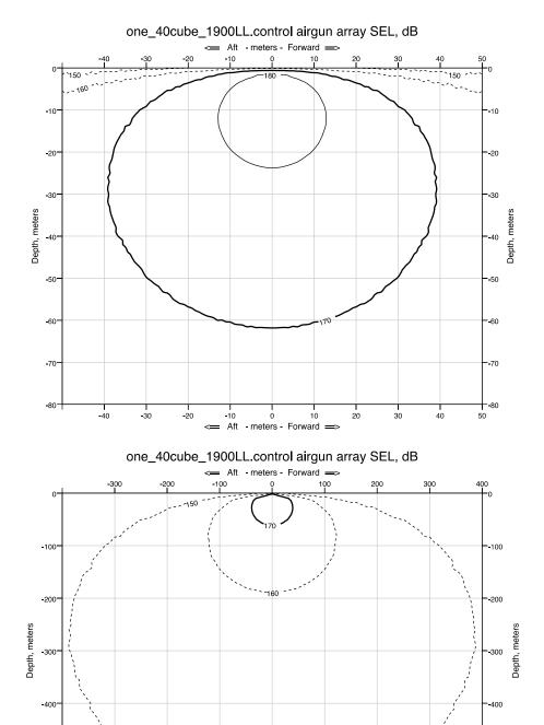
FIGURE A2. Modeled deep-water received sound levels (SELs) from a single 40-in<sup>3</sup> airgun towed at 9 m depth, which is planned for use as a mitigation gun during the proposed survey. Received RMS levels (SPLs) are expected to be ~10 dB higher. Plot at the top provides radius to the 170 dB SEL isopleths as a proxy for the 180 dB RMS isopleths and plot at the bottom provides radius to the 150 dB SEL isopleth as a proxy for the 160 dB RMS isopleth.
