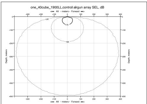
Figure 4 Modeled Deep-Water Received Sound Exposure Levels (SELs) from a Single 40-in<sup>3</sup> Airgun Towed at 9 Meters Depth
