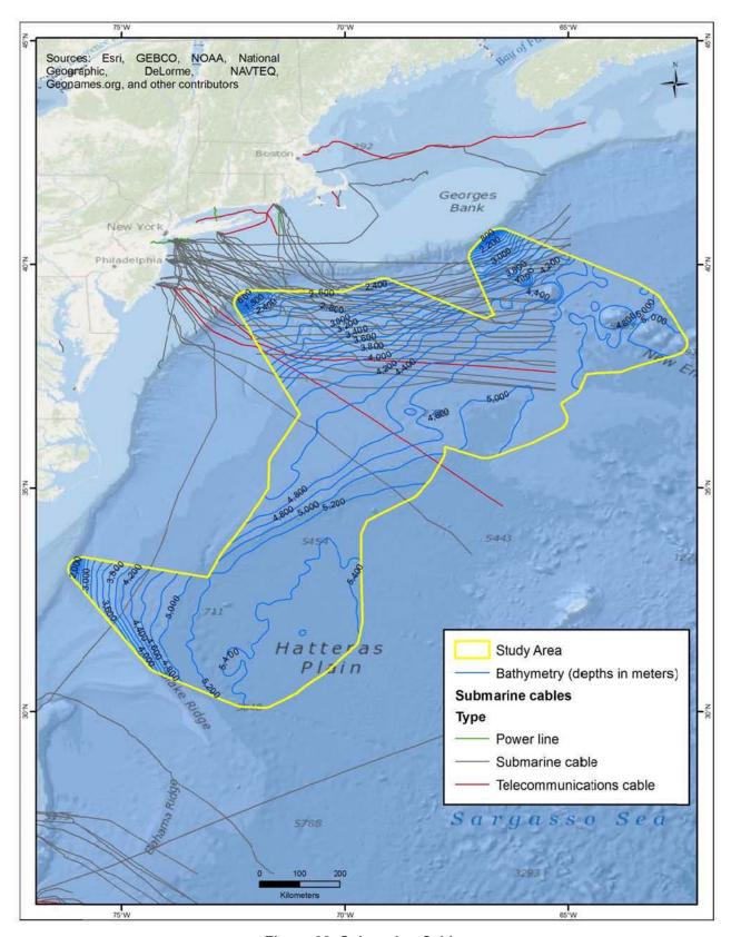
Figure 28: Submarine Cables
