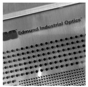
**Figure 19.** MI S/N 105 image of test target, taken during MER-2 system thermal testing.
