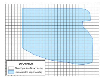
Step 2: Use a select by location tool to select the tiles that intersect with the lidar project boundary layer. Export the selected tiles to a new layer.
