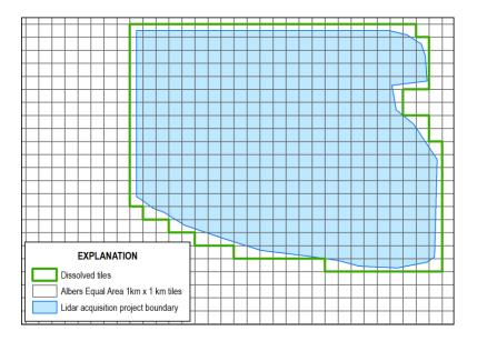
Step 4. Buffer the dissolved tiles polygon by 100 meters. (The 3DEP data processing workflow requires that all project boundaries include this buffer.) Ensure that the final project boundary is in the Albers Equal Area coordinate reference system (EPSG code 6350).
