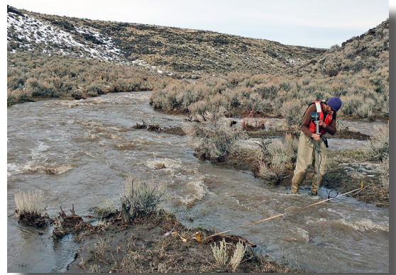
Measuring peak flow on Wickahoney Creek, February 2017 (Photo courtesy Bureau of Land Management)
