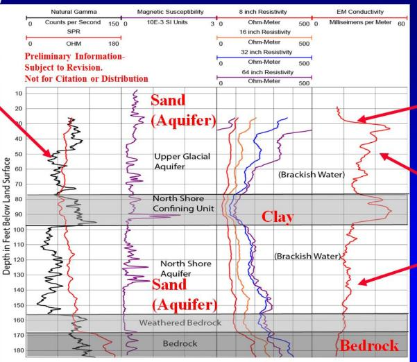
Suite of Borehole Geophysical Logs of Sands Point Outpost Well.
