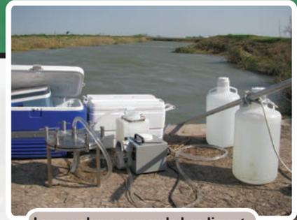
Large-volume suspended-sediment (LVSS) sampling equipment
