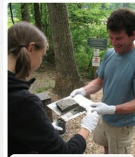
Subsampling a lake-bottom sediment box core
