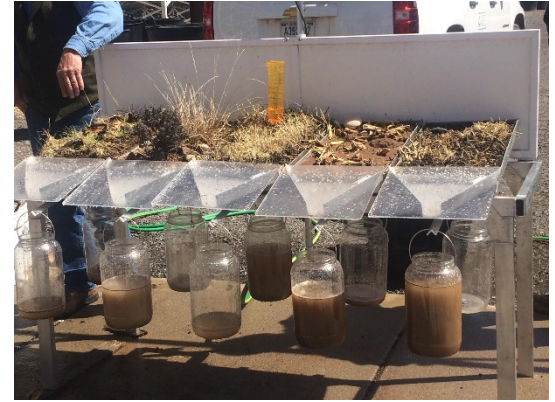
Natural Resource Conservation Service display illustrating effects of different soil-vegetation combinations on water runoff and absorption (Photo Credit: Molly McCormick, USGS)
