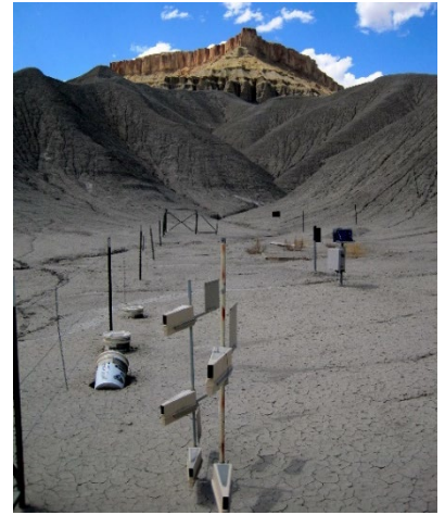
Dust samplers at a site in Utah are being used to help understand the transport of sediment via wind. (Photo credit: Erika Geiger, USGS)
