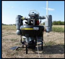
A new UAS, the T-Hawk, will be used during the next flights, along with new and improved cameras.
