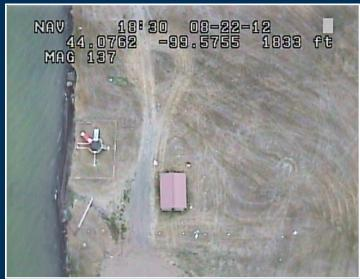
2012 flights documented that the bank had eroded, allowing the front of the wood frame and surrounding soil to disappear during the year around this playground equipment.
