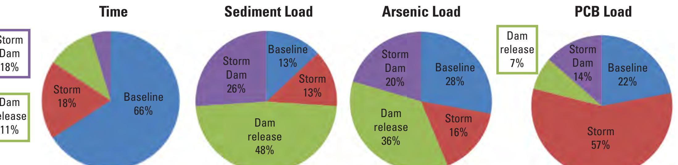
The pie charts show that most of the time the river is in a "baseline" condition, when sediment transport is low, and events that occur over a relatively short period of time make up the majority of sediment and chemical loads. However, the most chemical transport does not always coincide with the most sediment transport (dam releases).
