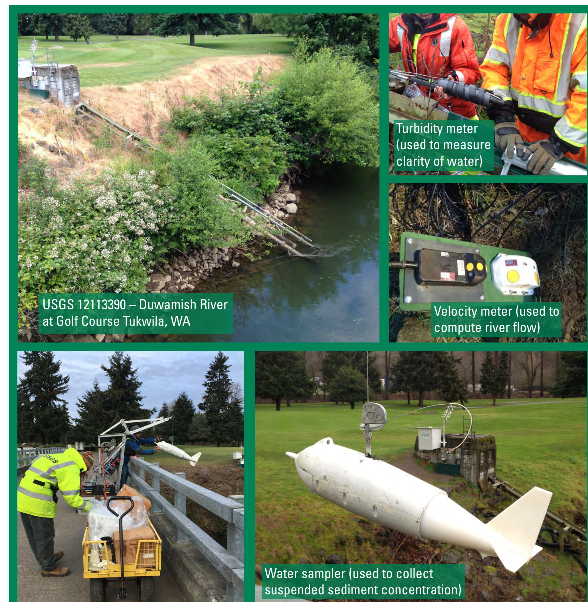
Turbidity (clarity or cloudiness of water, primary surrogate for suspended-sediment concentration) data were coupled with measured suspended-sediment concentration (particles of sediment suspended in water column, measured in milligrams per liter of water) to compute a record of suspended sediment concentrations. Discharge data were coupled with concentration data to compute total and fine particle suspended-sediment loads (mass per unit of time, that is concentration multiplied by river flow).
