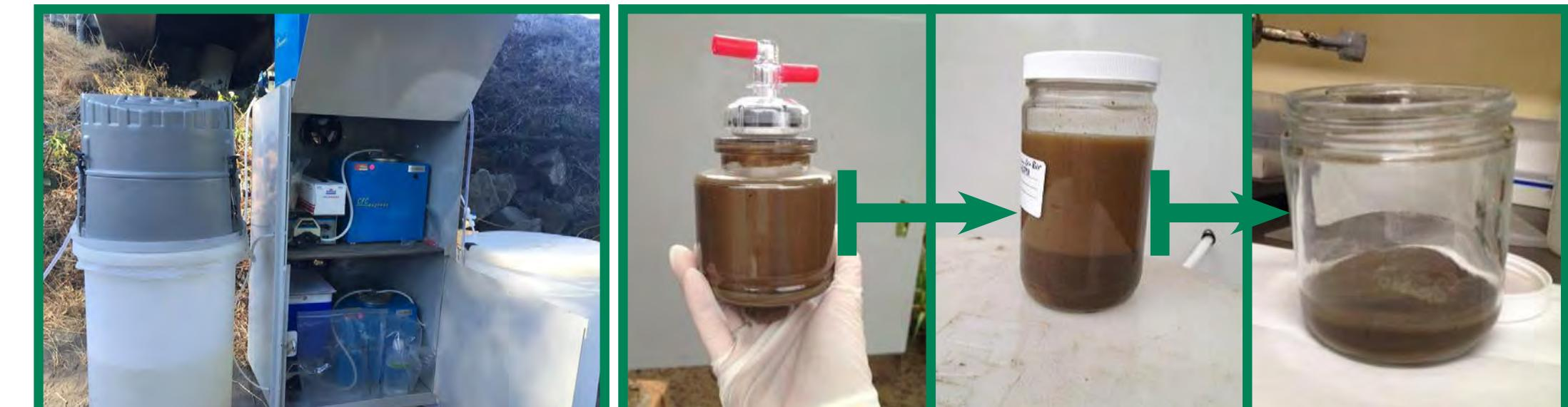
Chemicals such as metals and polychlorinated biphenyls (PCBs) were measured on suspended sediment using a novel field technique that separates suspended sediment from large volumes of river water using a continuous-flow centrifuge. (<https://www.youtube.com/watch?v=UuoIoyK3JIM>)
