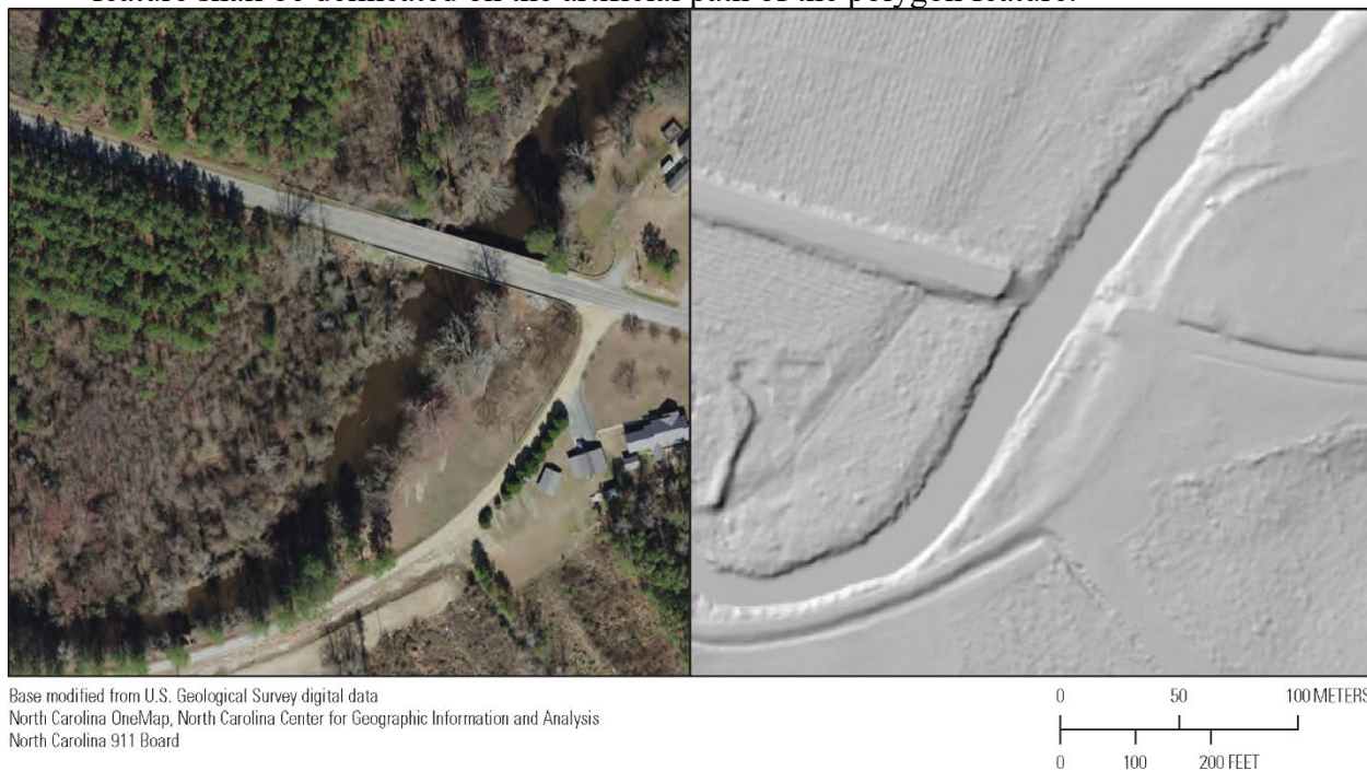
Figure 8. Bridge treatment in the bare-earth digital elevation model. The bridge deck is removed, and water surface is interpolated beneath the bridge to maintain a monotonic, continuous water feature.
