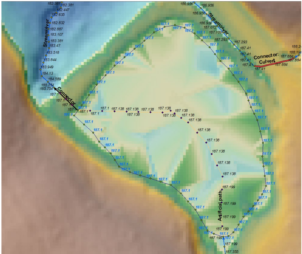
Figure 29. An example of an Artificial path feature maintaining downstream monotonicity. Z-values assigned to waterbody vertices are equal to the start node of the Connector feature at the outlet of the waterbody.
