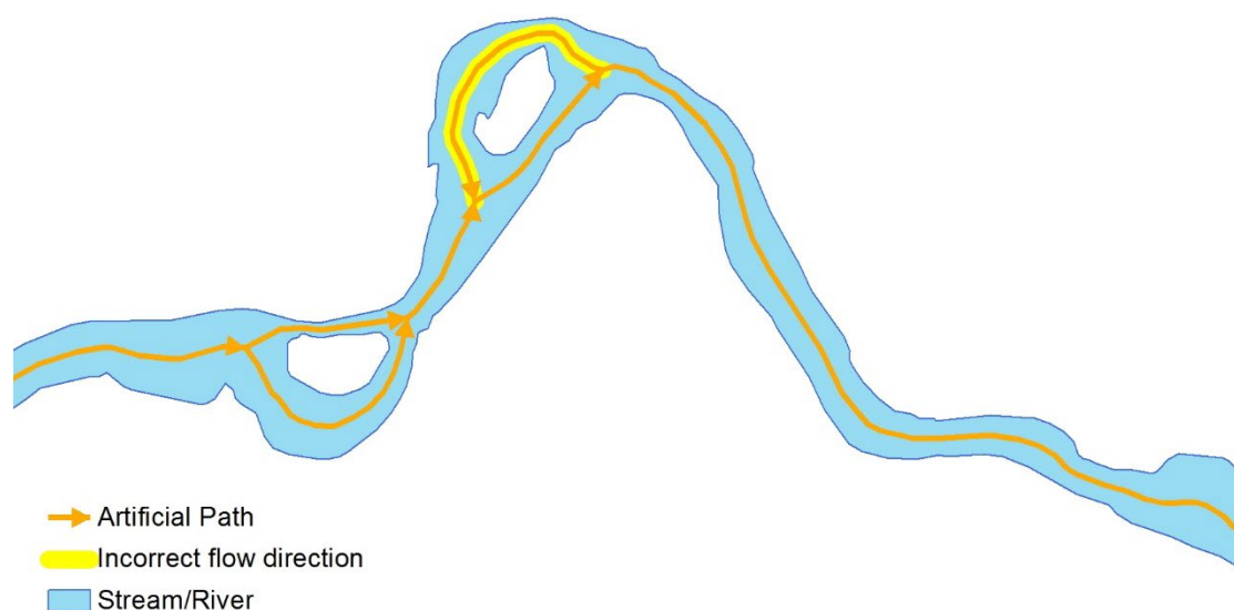
Figure 37. Lines shall always flow downstream monotonically. This example shows an incorrectly placed segment flowing upstream.
