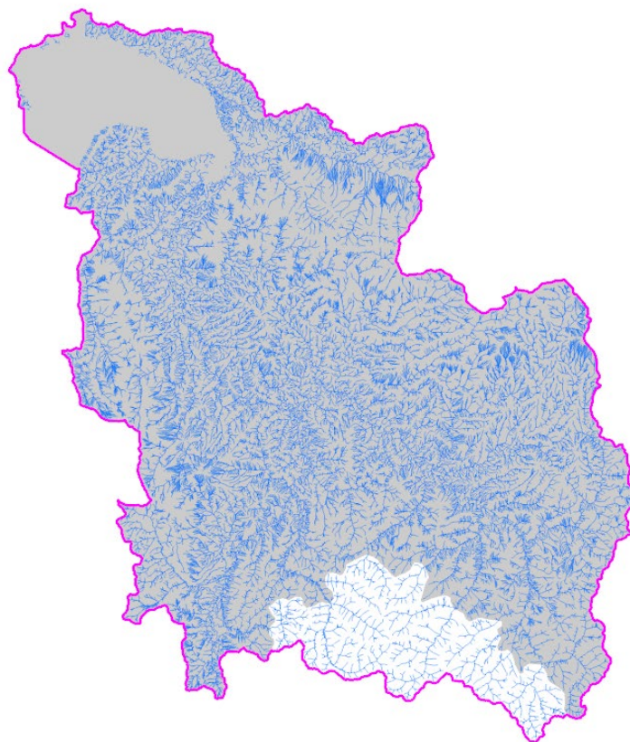
Figure 3. Final Deliverable Project Area (FDPA) (in magenta) encompassing additional elevation-derived hydrography contributing flow to the original Defined Project Area (DPA) (in gray).
