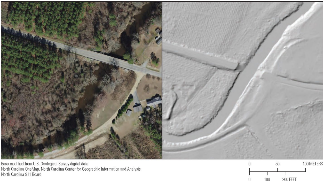
Figure 9. Bridge treatment in the bare-earth DEM. The bridge deck is removed, and water surface is interpolated beneath the bridge to maintain a monotonic, continuous water feature.
