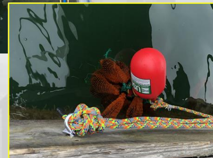
Sentinel Shellfish bags to monitor shellfish toxicity at Mount Desert Island Biological Laboratory, Maine.
