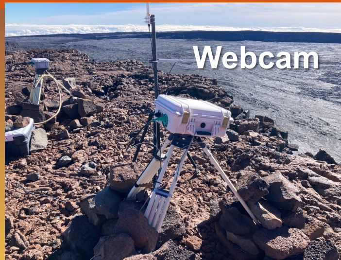
Telemetry hub and seismic station
