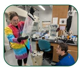
Top: The Algal and Environmental Toxins Unit is currently testing point-of-use drinking water treatment and filtration systems for the removal of algal toxins from freshwater sources.
