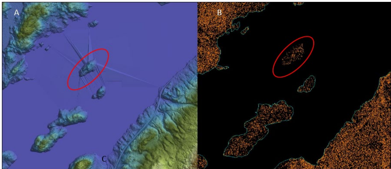
Figure 11. Digital elevation model (A) and classified lidar point cloud (B) showing an island (in red ellipse) that is classified correctly but is missing a breakline leading to an uneven water surface. The water surface should be flat. This island meets contracted minimum collection size for breaklines.
