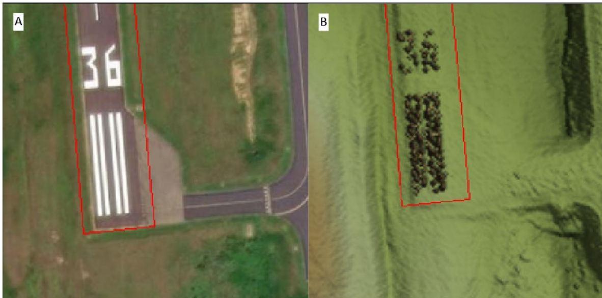
Figure 23. High noise from reflective surfaces on a runway (aerial photograph, A) have been left in the ground classification (digital elevation model, B).
