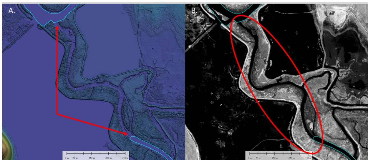
Figure 5. Digital elevation model (A) and intensity image (B) showing a discontinuous stream segment that should have been collected as a single water feature.
